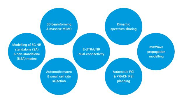
5G is a new paradigm for radio planning and optimisation activities, as huge amounts of predicted and live-network data need to be used for 5G network design. As an example, automatic planning and configuration of new cell sites in mmWave frequencies requires evaluating large numbers of candidates and generates intensive calculations to select best configuration parameters at the design stage.
